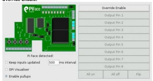
Toggle **Output Pin 1** on by clicking on it. The PiFace interface will click as the relay turns on and the corresponding LED will illuminate. Notice the graphic onscreen updates to show the LED being on, the contacts have changed over on the relay and the first output pin is on.
